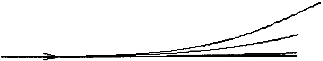
Fig.2. Trajectories after 1 second of flight for (top to bottom) \lambda = 0, 0.001, 0.01, 1 . For \lambda = 1 , the horizontal distance traveled is 288 \text{ m} .
