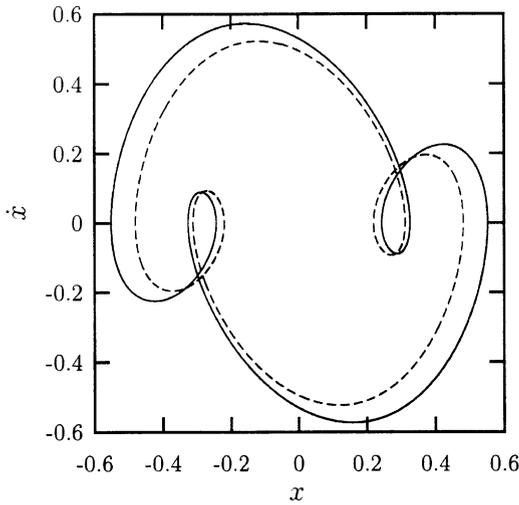
Fig. 5. Comparison of numerical and analytical approximations of the unstable periodic orbit in the phase plane. Analytical approximation is dashed, numerical integration is solid. Here  $\delta = 0.631$ ,  $\varepsilon = 1.47$  and  $A = 0.3811$ .  $\delta_0 \approx 0.6304$  and  $\varepsilon_0 \approx 1.4386$ .
