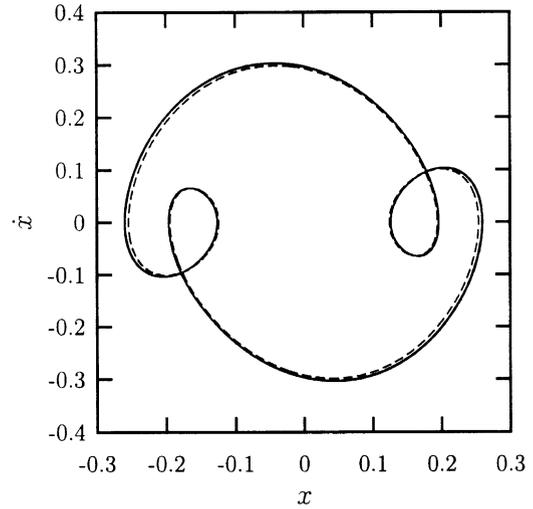
Fig. 3. Comparison of numerical and analytical approximations of the unstable periodic orbit in the phase plane. Analytical approximation is dashed, numerical integration is solid. Here  $\delta = 0.6305$ ,  $\varepsilon = 1.47$  and  $A = 0.2542$ .  $\delta_0 \approx 0.6304$  and  $\varepsilon_0 \approx 1.4386$ .
