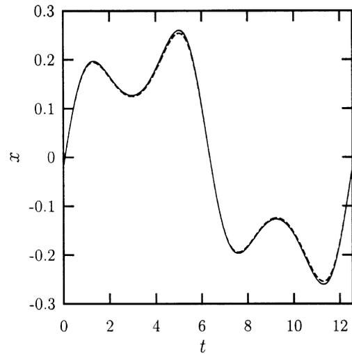
Fig. 4. Comparison of numerical and analytical approximations of the unstable periodic orbit as a time history. Analytical approximation is dashed, numerical integration is solid. Here  $\delta = 0.6305$ ,  $\varepsilon = 1.47$  and  $A = 0.2542$ .  $\delta_0 \approx 0.6304$  and  $\varepsilon_0 \approx 1.4386$ .
