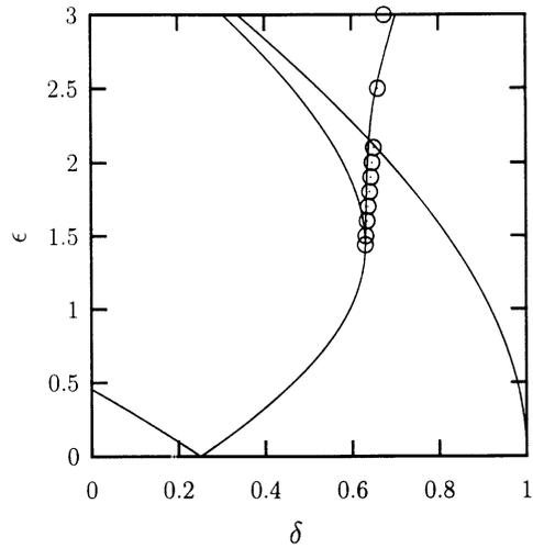
Fig. 7. Comparison of analytical and numerical approximation to the secondary bifurcation curve. Analytical approximation is the solid line, numerical values are points.
