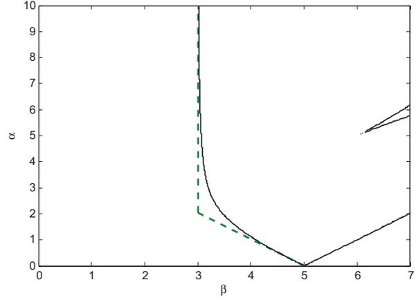
Fig. 5. LINEAR PIECEWISE APPROXIMATION FOR THE DRIFT/LOCK BOUNDARY.  $\Omega_2 = 5$ .
