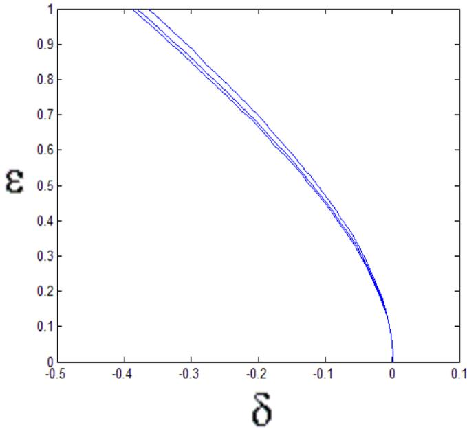
Figure 5.  $n = 0$  transition curve, eq.(54), in the fractional Mathieu equation (38) for  $c = 0.1$  and  $\alpha = 0, 0.5, 1$ . The leftmost curve corresponds to  $\alpha = 0$ . The middle curve corresponds to  $\alpha = 0.5$ . The rightmost curve corresponds to  $\alpha = 1$ .
