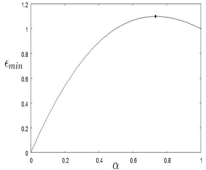
Figure 7. Plot of  $\epsilon_{min}$ , the minimum quantity of forcing amplitude  $\epsilon$  necessary to produce instability, as a function of fractional derivative order  $\alpha$ , eq.(55). The greatest effect is observed where this curve achieves its maximum, shown as a dot here, and referred to as  $\alpha^*$  in the text.
