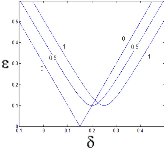
Figure 3.  $n = 1$  transition curve, eq.(51), in the fractional Mathieu equation (38) for  $c = 0.1$  and  $\alpha = 0, 0.5, 1$ .
