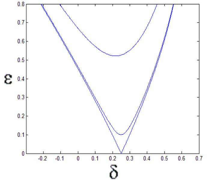
Figure 2. Transition curves (37) in the damped Mathieu equation (36). The upper curve corresponds to  $c = 0.5$ . The middle curve corresponds to  $c = 0.1$ . The lower curve corresponds to  $c = 0$ .
