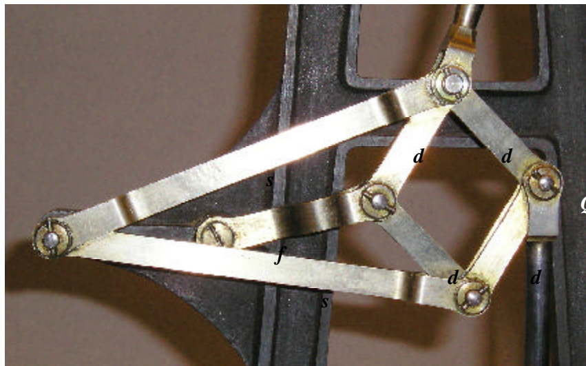
Figure 1.5 Peaucellier/Lipkin linkage for drawing a straight line
